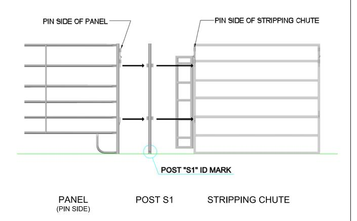
PANEL TO STRIPING CHUTE CONNECTION w/ POST S1
