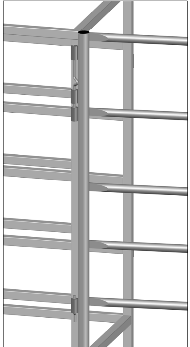
PANEL TO REAR OF STRIPPING CHUTE (PIN TO SPOOL)
