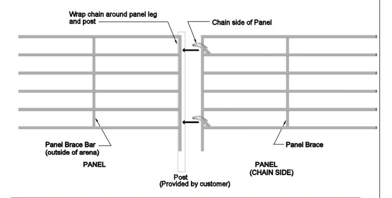
NOTE: IF USING PUT-10 or PL SERIES PANELS THE PANELS VERTICAL FITTED BRACE BAR FACES INSIDE OF THE ARENA AREA
