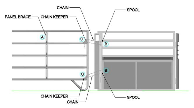
PANEL w/ DBL CHAINS (CHAINS ON BOTH SIDES OF PANEL) ROPING CHUTE RIGHT SIDE
