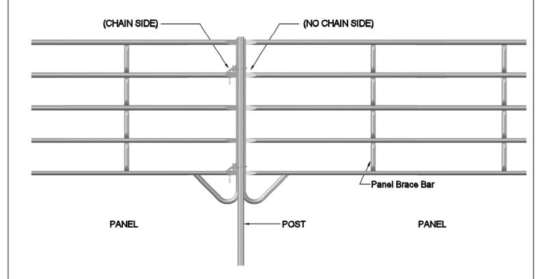
NOTE: WHEN PLACING PANELS - THE PANEL BRACE BAR FACES INSIDE OF THE ARENA AREA AND POST ARE OUTSIDE OF ARENA
