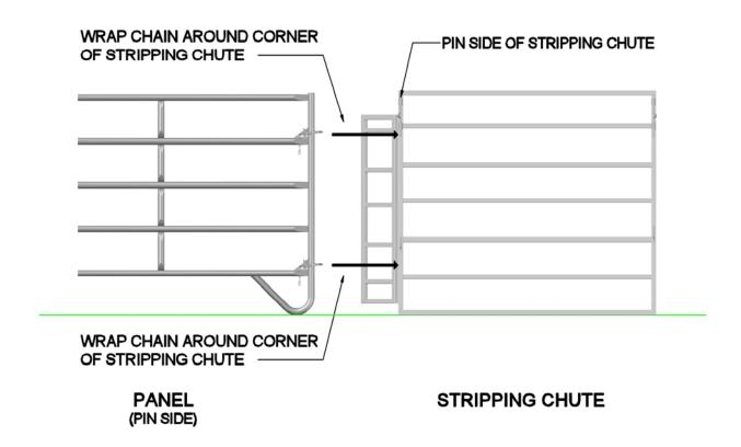
PANEL TO STRIPING CHUTE CONNECTION
