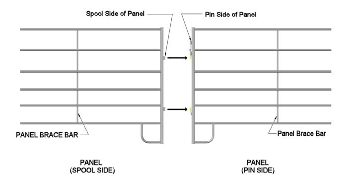
NOTE: WHEN PLACING PANELS - THE PANEL BRACE BAR FACES OUTSIDE OF THE ARENA AREA
