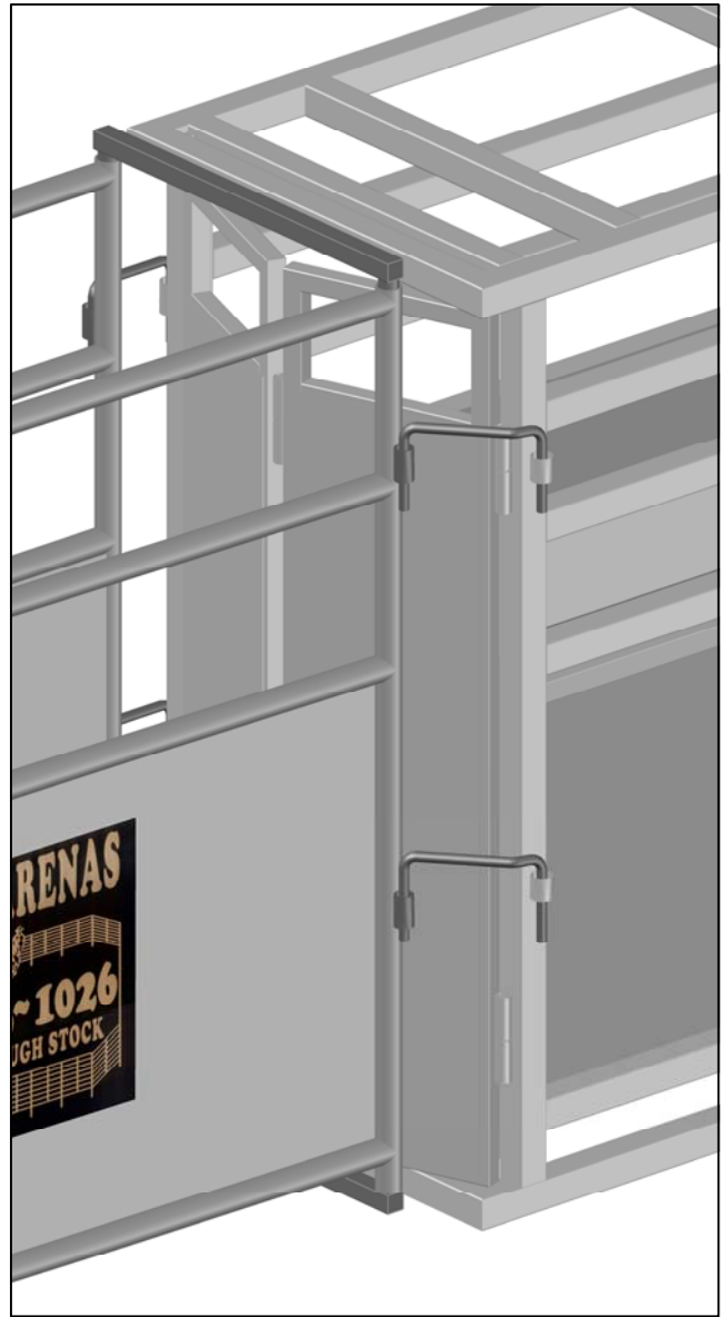
ROPING CHUTE RIGHT SIDE (1/2" x 8" BENT U-BAR)
