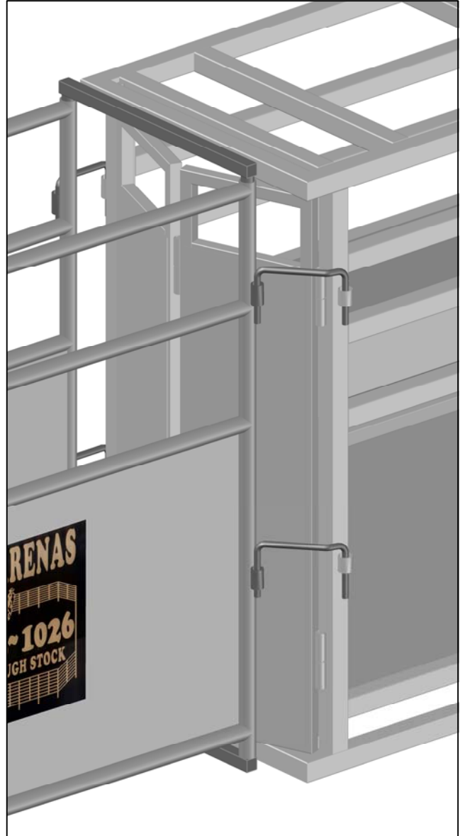
ROPING CHUTE RIGHT SIDE (5/8" x 8" BENT U-BAR)
