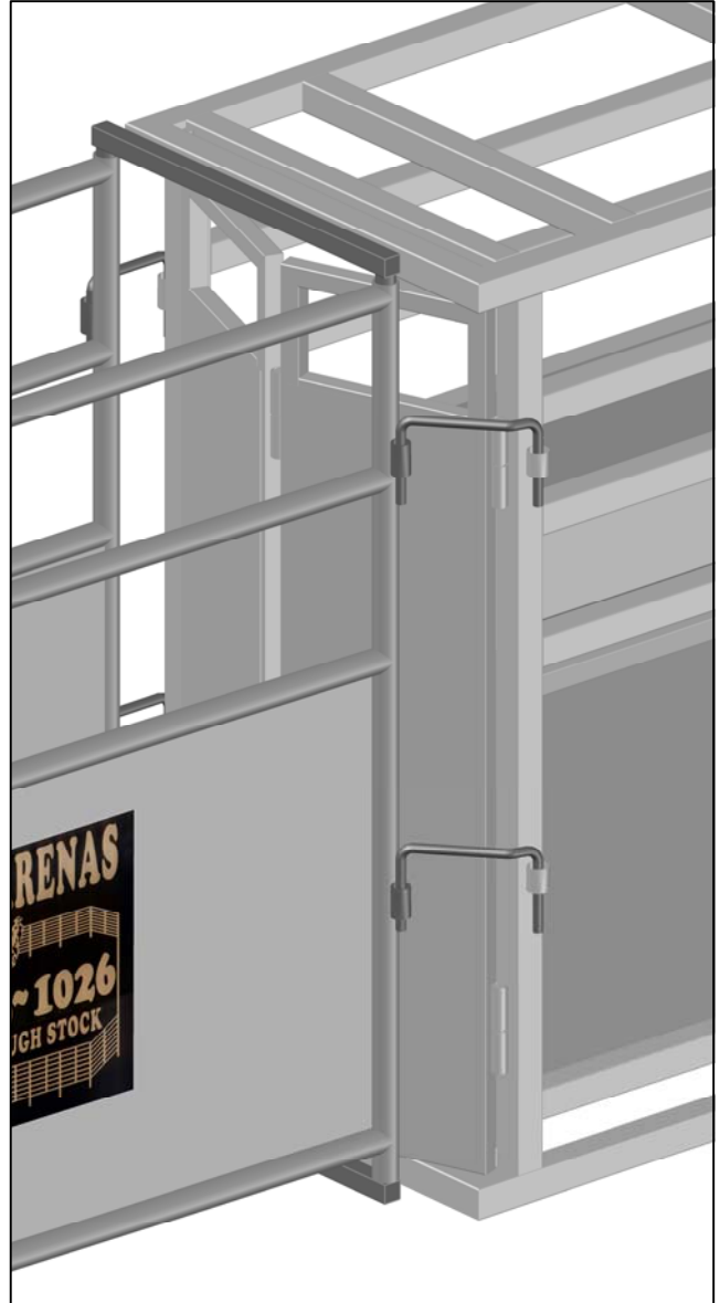
ROPING CHUTE RIGHT SIDE (5/8" x 8" BENT U-BAR)
