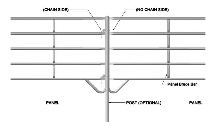
NOTE: WHEN PLACING PANELS - THE PANEL BRACE BAR FACES INSIDE OF THE ARENA AREA AND POST ARE OUTSIDE OF ARENA
