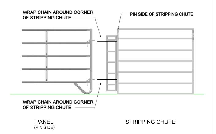
PANEL TO STRIPING CHUTE CONNECTION w/ POST S1
