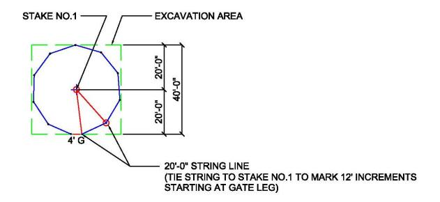
NOTE: STARTING AT THE GATE, USE THE 20' STRING LINE AND STEP 12' TO MARK A PANEL POINT USING SPRAY PAINT, POWDER OR FLAGS WILL GIVE YOU ESTABLISHED POINTS AS A GUIDE LINE.
