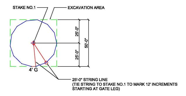
NOTE: STARTING AT THE GATE, USE THE 25' STRING LINE AND STEP 12' TO MARK A PANEL POINT USING SPRAY PAINT, POWDER OR FLAGS WILL GIVE YOU ESTABLISHED POINTS AS A GUIDE LINE.
