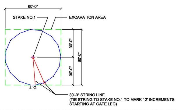
NOTE: STARTING AT THE GATE, USE THE 30' STRING LINE AND STEP 12' TO MARK A PANEL POINT USING SPRAY PAINT, POWDER OR FLAGS WILL GIVE YOU ESTABLISHED POINTS AS A GUIDE LINE.
